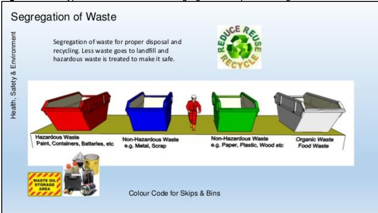
Figure 2 Typical construction waste segregation compound design
